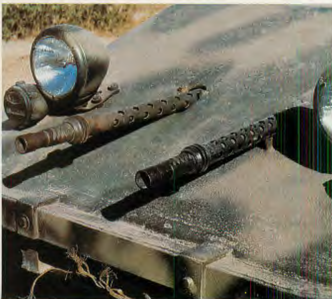
BELOW: Twin fifties in front hull of M114 track. Gun on the right is non-functional as driver sits directly to the rear of it.
